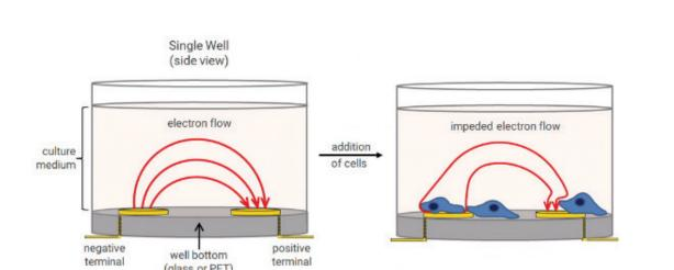
Microelectrodes fused to the bottom of a microtiter plate measure the presence of adherent cells which impede electron flow. Impedance is reported as cell index (CI) which increases as cells proliferate.
