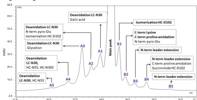
**Fig. 9** CEX-HPLC chromatogram of in-house IgG1 mAb showing acidic and basic product related variants.
