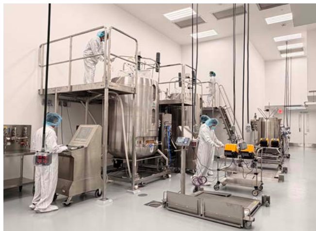
Figure 1. Newly installed 2,000L single-use bioreactors successfully completed initial engineering campaign following site expansion.
